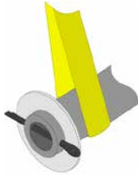
Fig. 7 Detail of hooking the sling to the lifting tube
