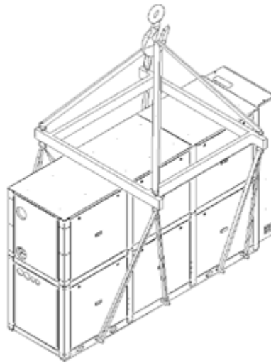
Fig. 8 Lifting with crane
